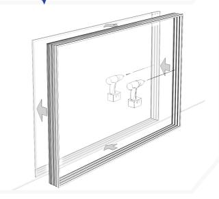
Make a small sealing in the corners to make sure that no water is able to run through the conection.
